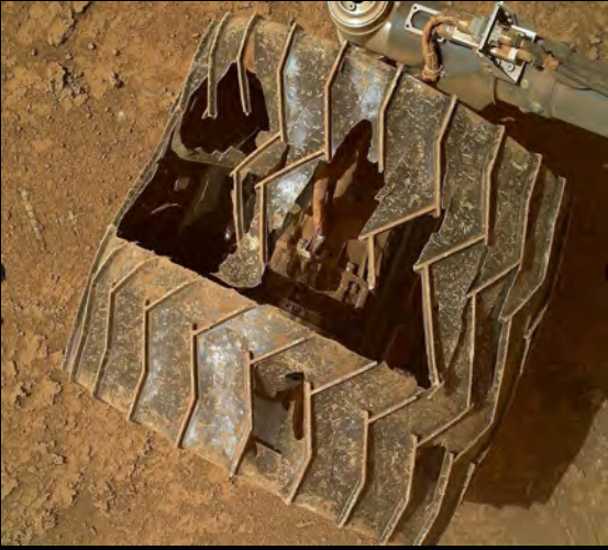
MARS Curiosity Rover wheel driven 22+ miles since 2012
